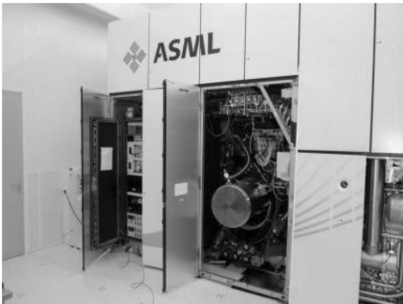
Figure 3: HVM I LPP Source Vessel Integrated into the NXE 3100 Scanner.
