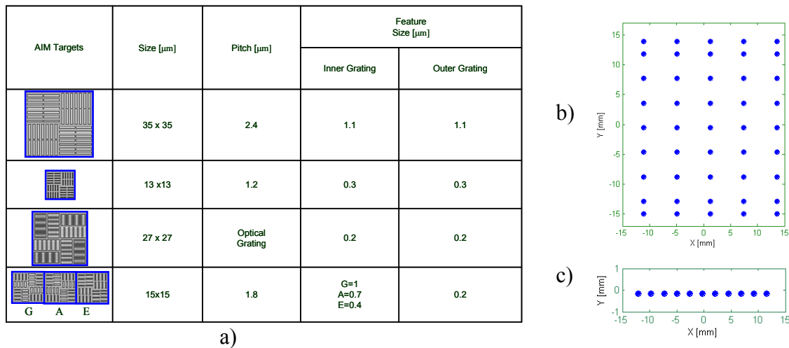
Figure 13: starting from the top: the first 3 rows are AIM targets used for distortion calculation, 2-pass overlay test. The last row shows targets {G, A, E} which are suitable targets to evaluate the imaging fingerprint across the slit. b) Field sampling for 2-pass overlay test. c) Slit sampling for IPE calculation
