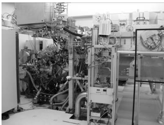
Figure 6: Prototype LPP source integrated with the mid frame vessel.
