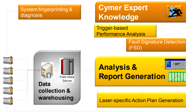
Figure 8 – Down time reduction through automation of data analysis of light source performance data. Centralized data collection and warehousing enables the use of fault signature detection (FSD) to automate knowledge derived from laser experts, which can trigger a scheduled maintenance action. Continuous diagnostics generation shortens or eliminates the time required to troubleshoot a fault.
