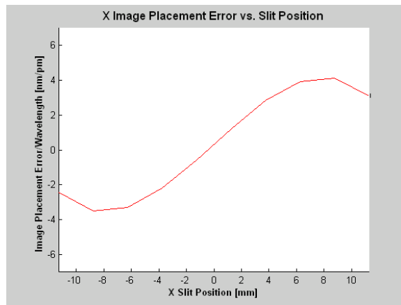
Figure 21. IPE rate of change as a function of slit position for the 193nm lens.
