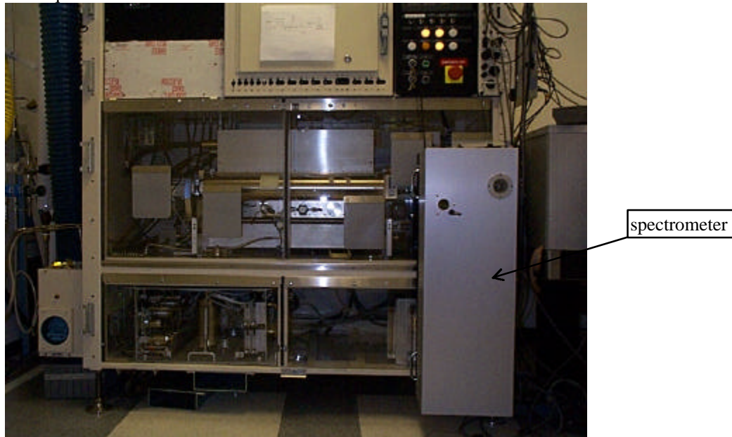
Fig. 5. Compact high resolution grating spectrometer shown installed on Cymer ELS-5000 KrF excimer laser.
